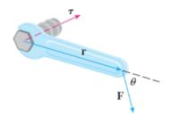
Example: A wrench 30cm long lies along the positive y-axis and grips a bolt at the origin. A force is applied in the direction (0, 3, -4) at the end of the wrench. Find the magnitude of the force needed to supply 100N·m of torque to the bolt.
